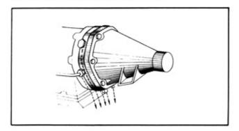
Fig. TM-5 Oil leak point of rear extension
