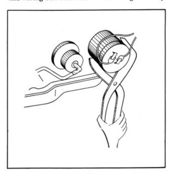
Fig. TM-6 Removing downshift solenoid
