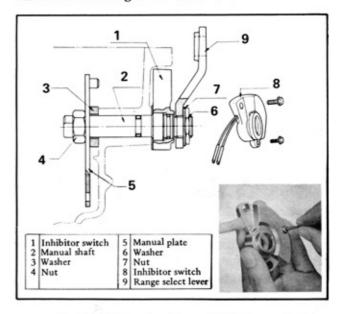
Fig. TM-8 Construction of inhibitor switch
