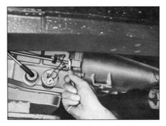
Fig. TM-12 Removing oil cooler tube
