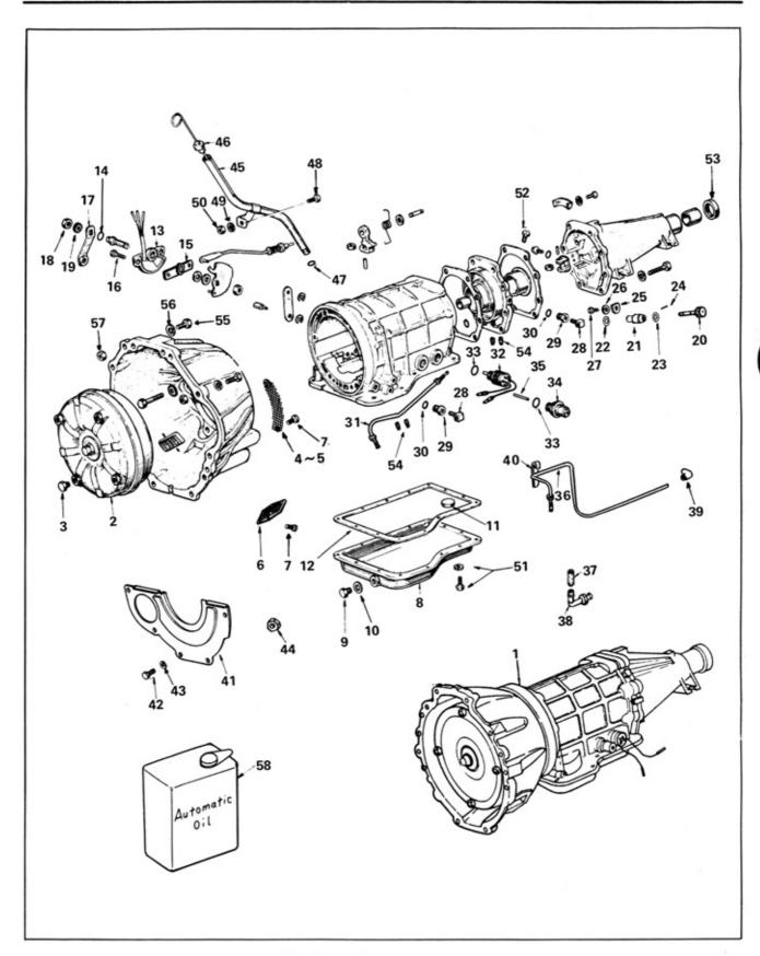
Fig. TM-2 Transmission case
