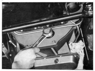
Fig. TM-13 Removing torque converter fixing bolt
