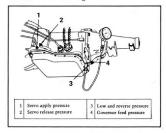
Fig. TM-9 Measuring line pressure
