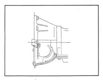
Fig. TM-4 Oil leak point of converter housing
