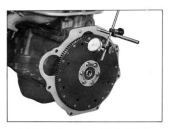
Fig. TM-14 Checking run-out of drive plate
