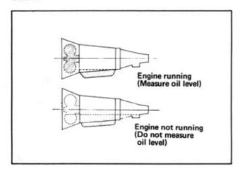
Fig. TM-3 Measuring oil level
