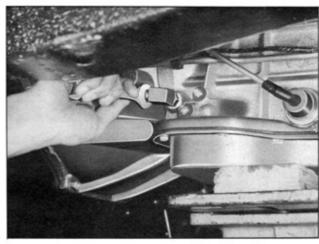
Fig. TM-11 Removing oil cooler tube
